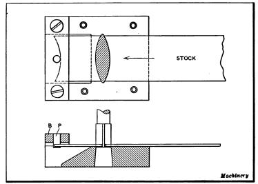
Fig. 32. Stop-pin of the Bridge Type
